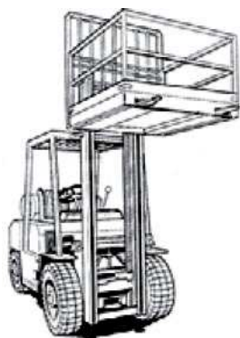
Figure 1 Counterbalance truck with non-integrated working platform
